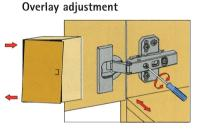
Turn screw clockwise: Door overlay decreases (-). Turn screw anticlockwise: Door overlay increases (+).
